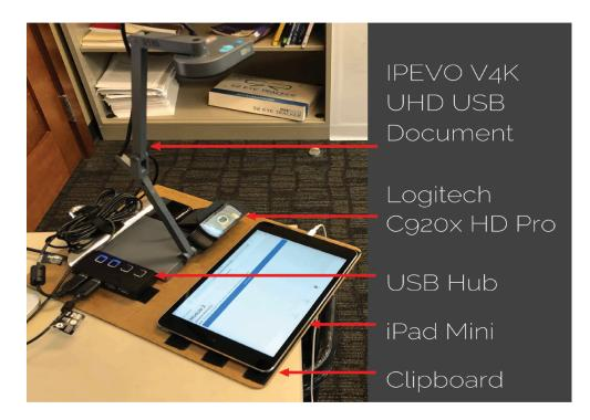
This hardware configuration uses a USB document camera to record the screen of the mobile device, which allows for capturing finger movements and gestures. It also uses a webcam to record the user. These devices are connected to a USB hub, which is connected to a laptop running OBS Studio (Figure 5).
